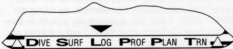
Figure 2: The Mode Indicator makes it easy to determine which mode the AWAC-1 is currently displaying.
