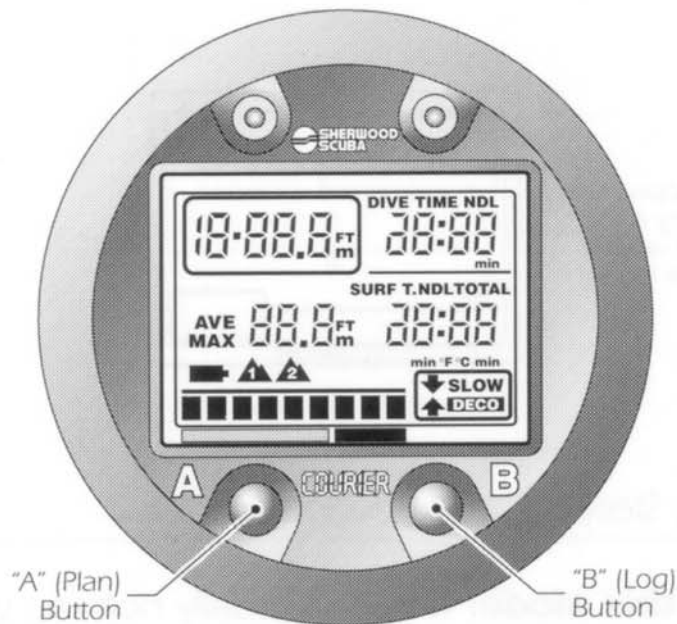
Figure 1: The front of the Courier, showing its Liquid Crystal Display (LCD) in Check Mode, and the two large A (Plan) and B (Log) buttons.
