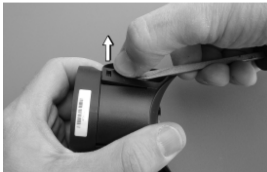
Fig. 14 – Exhaust Tee Removal - Step 1
