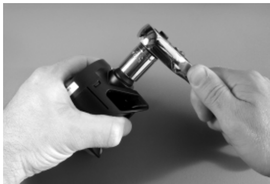
Fig. 23 – Packing Nut Installation
