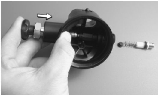
Fig. 9 – Adjustment Stem Removal
