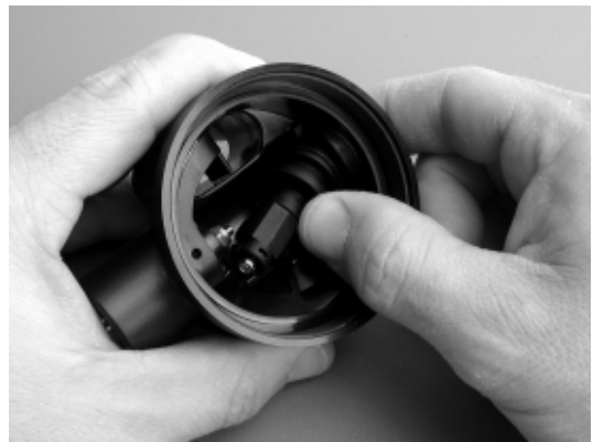
Fig. 11 – Adjustment Tube Removal
