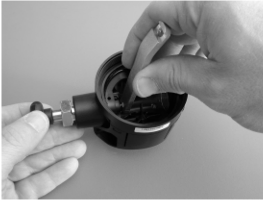
Fig. 13 – Disassembly of Poppet
