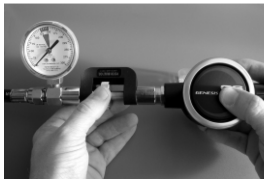
Fig. 27 - Inline Adjustment Tool w/ IP Gauge
