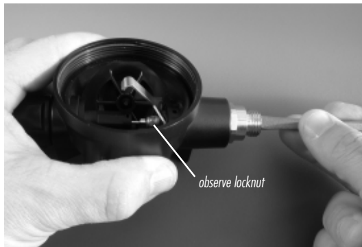
Fig. 25 – Orifice Preliminary Setting
