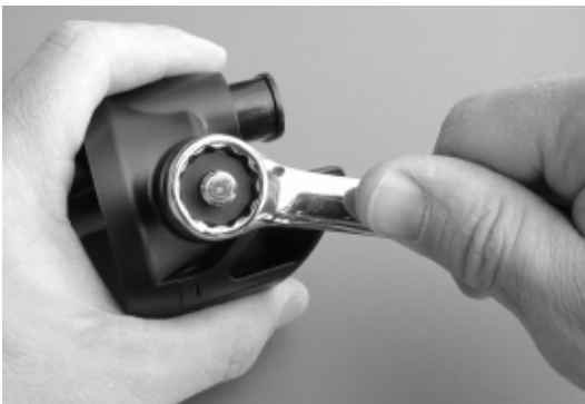
Fig. 8 – Packing Nut Removal
