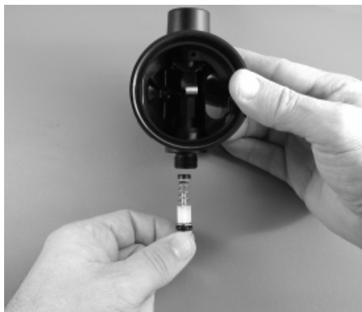
Fig. 22 – Adjustment Stem Installation
