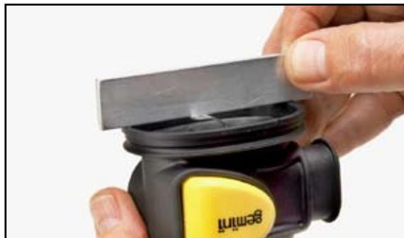
*Lever height adjustment even with edge of housing*
