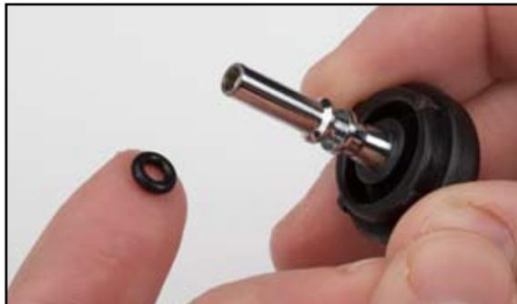
*Slide o-ring over shaft and seat in groove.*
