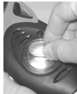
Fig. 80 - Battery Hatch Removal
