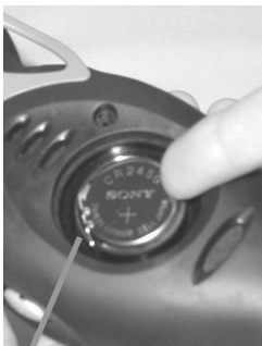
a Fig. 82 - Battery Installation
